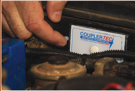
▲ We fitted 6 charge pads to the cruiser's bodywork.
