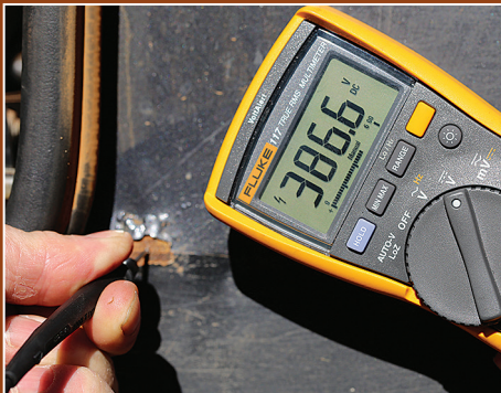
▼ Testing a monitored rust patch showed a high voltage cancelling electron loss.
