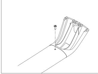
Insert the rubber buffer strip into the top of the crossbar.
