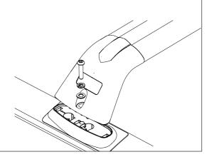
Insert the screw assembly into the support leg mounting holes. Using the allen key provided tighten the support leg screws to secure the crossbars. Recommended tightening torque 4N/m. DO NOT OVER TIGHTEN.
