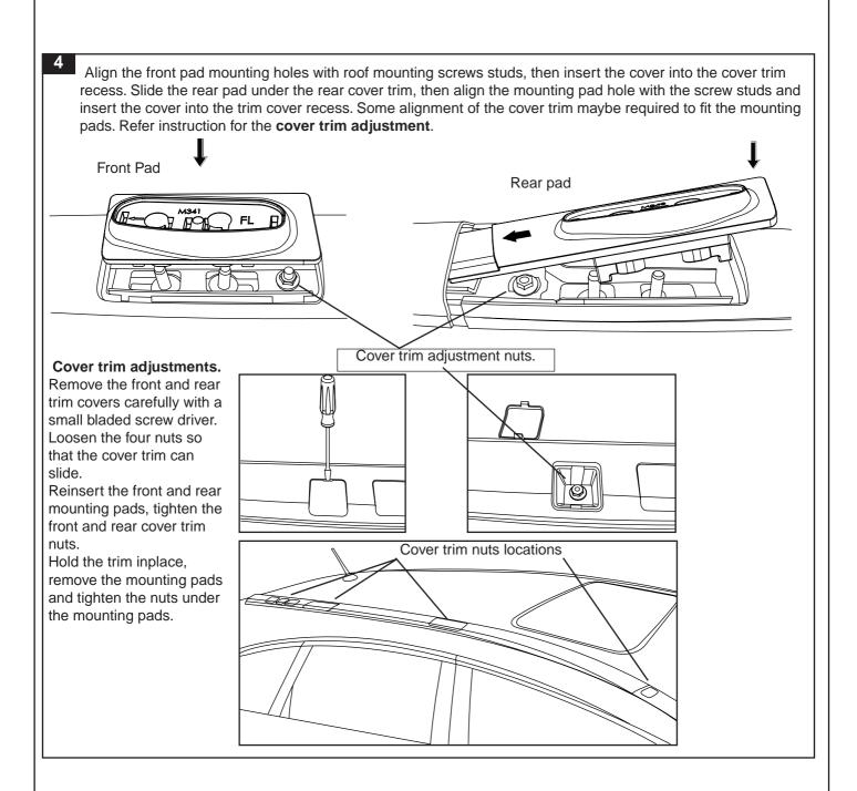
Insert the tube nuts into the pad mounting holes and using the allen key carefully tighten. Recommended tightening torque 4N/m. **DO NOT OVERTIGHTEN.** Repeat this process for each of the four pads.
