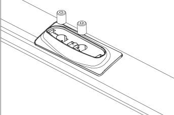
Insert the support leg fully into the crossbars, a rubber mallet may be required to knock the leg in place.
