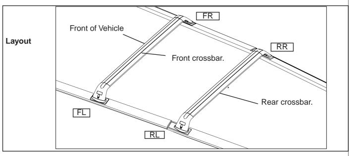
Remove the four covers from the roof rack mounting locations by carefully inserting a small bladed screwdriver into the cut outs in the front and rear covers and lever downwards carefully.
