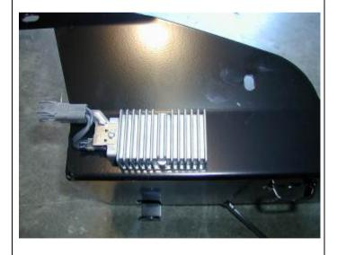
5. On V6 petrol models attach the module removed in the step 3 to the side of the battery tray using the original screws.
