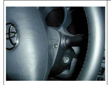
23. Remove the lower trim from the steering column. To do this turn the steering wheel 90 degrees and remove the two screws on the face of the trim. Also remove the screw on the lower part of the trim. Carefully remove the bottom half of the steering column trim.
