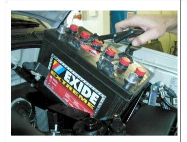
19. Place the battery in the tray by tilting it towards the front of the vehicle.
