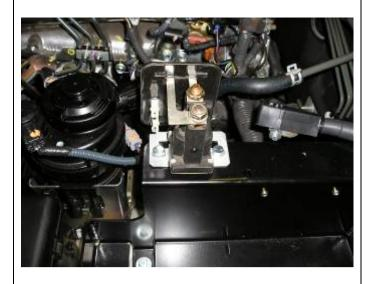
13. Attach the battery separator to the battery tray using two M6 x16mm bolts, M6 flat washers and M6 flange nuts.
