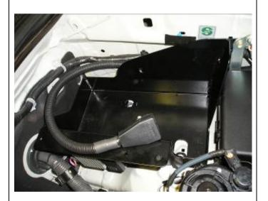
12. Run the earth cable (part No 6821125) behind the battery tray.
