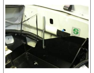
18. Place the 135mm L-bolt into the hole on the outside edge of the battery tray. Use a piece of tape to hold the L-bolt in place.
