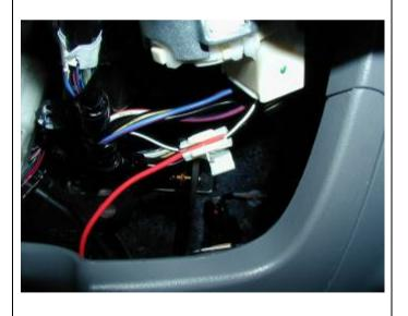
24. Connect the start assist wire to the vehicles starting wire in the steering column (black with a white trace, check with a test light first) using the scotch lock provided. Re-assemble the steering column trim.
