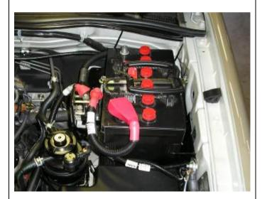
20. Connect the short positive cable (part No 6821103) between the auxiliary battery and the separator and the long positive cable (part No 6821139) between the main battery and the separator.
