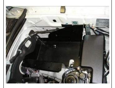
7. Place the battery tray in the engine bay ensuring that the tag on the side of the battery tray sits behind the earth bracket.
