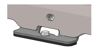
20. With assistance, carefully place the BASERACK on the vehicle so the inside of the blade brackets rests on the outside of the mounting brackets. The entire BASERACK assembly should be clear of the vehicle roof. All mounting holes/slots should align closely.
