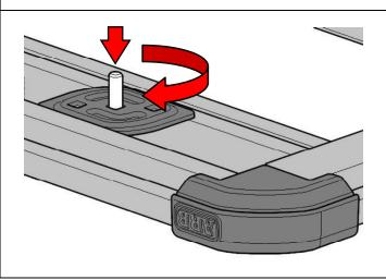
14. Flip the plate over and insert each of the assembled stud plates into the front channel of the BASE RACK.
