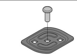
13. Insert one M8 x 20 Stud into each of the Stud Plates as shown.
