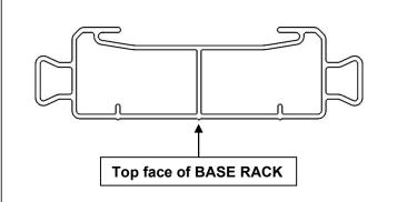
Place the BASE RACK face down on a clean flat surface. Provide protection to the top face of BASE RACK to avoid marking of surfaces
