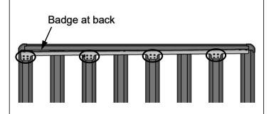
Check the position of the mounting plates (circled in image) on the blade brackets in relation to the channels on the BASE RACK.
