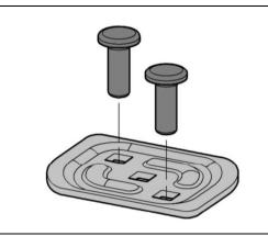
6. Insert 2, M8 x 20 Studs into each of the Stud Plates as shown.
