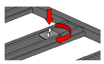
7. Insert the assembled stud plates into the correct BASE RACK channels. Rotate the plates 90 degrees.
