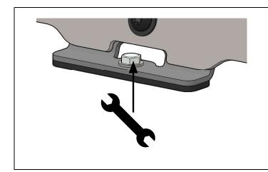
24. **If needed**, loosen M6 Hexagonal screws of misaligned mount brackets.
