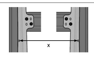
Using the previously recorded measurements, adjust the location of the blade bracket on the BASE RACK.
