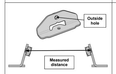
3. Using a tape measure, measure across the vehicle between the middle of the hole on the outside face of the front and rear set of mounting brackets. Make a note of each measurement.
