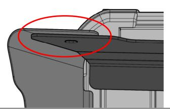
15. Position the air deflector on the BASE RACK with the M8 studs in the slots.
