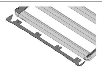
Note: BASE RACK should be upside down with the vehicle mount brackets fitted.
