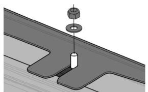
16. Attach the air deflector mounting slots to the stud plates with an M8 flat washer & nyloc nut.
