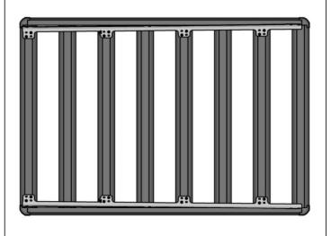
8. Flip the blade brackets over so they are upside down and carefully place on top of the BASE RACK. Ensure the M8 studs go through the slots.
