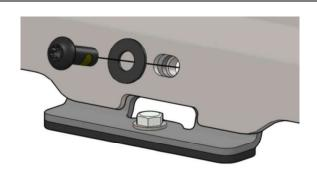
22. Use the M8 Button head Torx screws and M8 Black washers to secure the roof tray to the roof mounting brackets. Tighten all screws to the specified torque.
