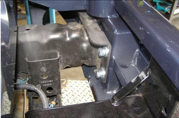
10. Loosely fasten bull bar to vehicle chassis using M10 fasteners supplied in chassis mounting kit.
