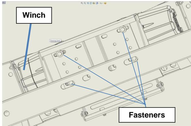
16. Lower winch onto bull bar mounting platform carefully aligning with slots.
