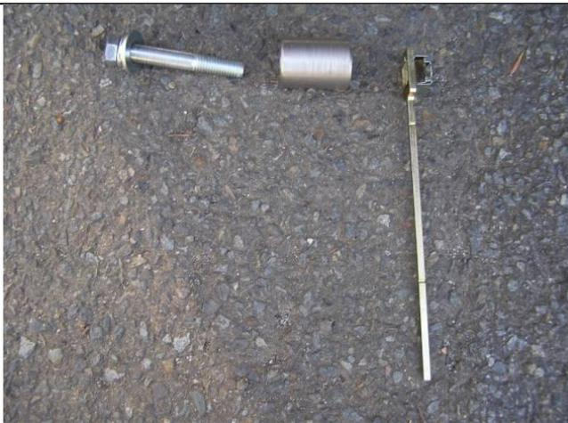
12. Position packers in between bull bar mounting bracket and chassis (at rear most slot in bracket).
