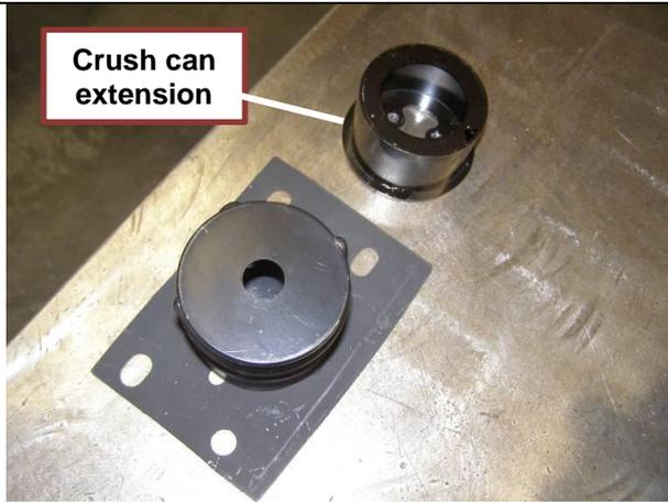
3. Attach crush can extensions supplied with bull bar to crush cans using 6x self-drilling screws supplied with crush can extension fitting kit **ACCESSORY Part No 3550140** (3x screws per crush can).
