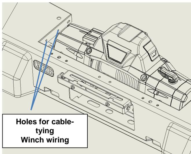
17. Use cable ties to fix winch power cables to pan to tidy up area.
