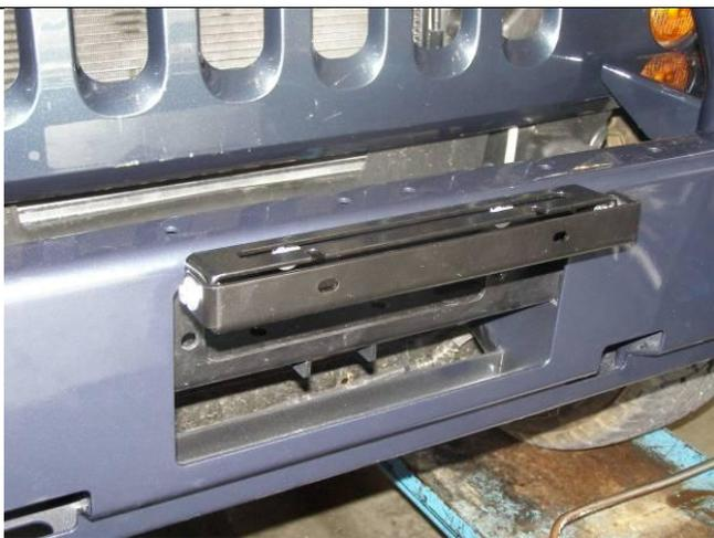
15. Mount number plate bracket assembly to bull bar using M6 fasteners supplied with number plate fitting kit.
