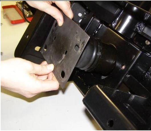
9. Position crush cans into mounting bracket openings located at the rear of the bar.
