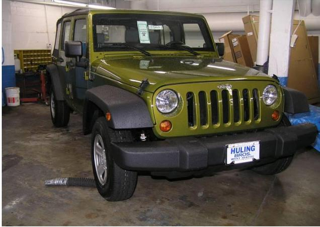
1. Remove plastic bumper from the vehicle including all hardware located behind it.
