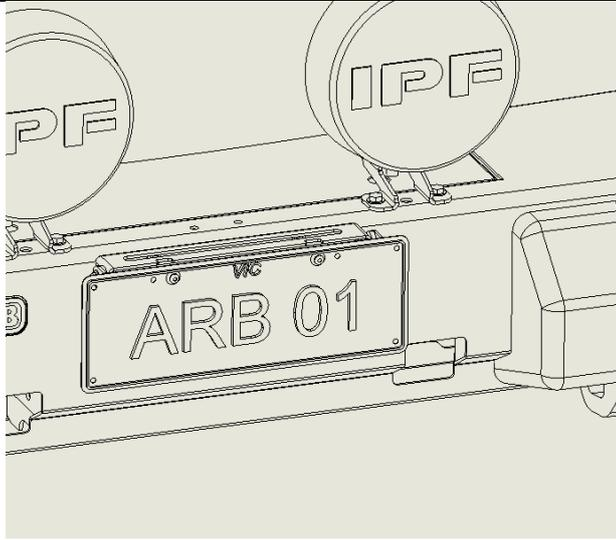
24. Bolt number plate to number plate bracket using M6 fasteners supplied with number plate assembly kit.
