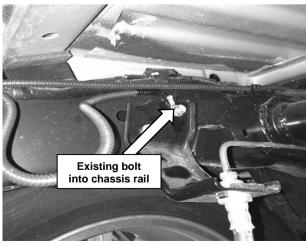
16. Connect the ground wire of the RSTB harness to the bolt on the LH chassis rail located in front of the rear cross member near the brake line mount.
