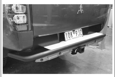
63. Attach the step plate extrusion to the RSTB using 8 M6x1.0x16 button head screws. Tighten fasteners to the specified torque.
