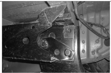
Remove bolt plate from inside of chassis rail from each side and discard as shown and remove bumper bar
