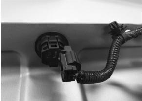
57. Clip the inner sensor into the housing as shown
