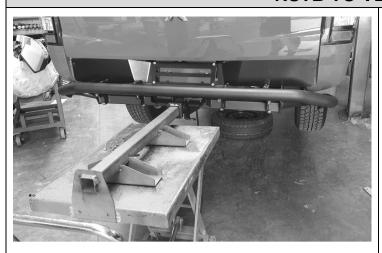
With the assistance of other people or a lifting device, lift the RSTB up beneath the chassis rails aligning the holes in the side of the chassis with those in the vertical surfaces of the RSTB.
