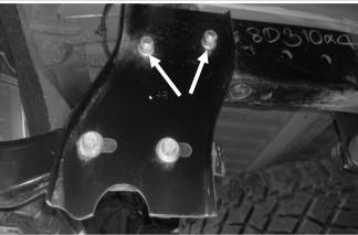
2. Remove licence plate and disassemble the bumper bar from the chassis by removing 2 M12 nuts from each side as shown.
