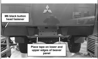
36. Attach beaver panel to rear of tub as shown using single M6x1.0x16 black button head fastener with black flat washer, M6 nyloc and flat black washer on tub inside face
