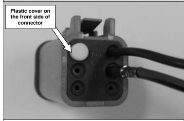
10. Insert one set of wires into a male 6-pin connector from the back in the following order:
