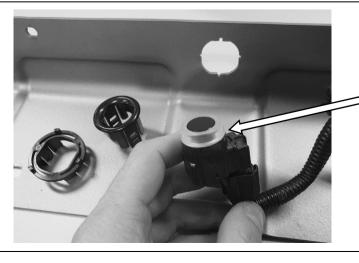
55. Remove the OE silicone sleeves on each sensor and replace with the thicker ones supplied with the fitting kit.
