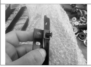
38. Insert canoe clip into both LH and RH number plate mount brackets as shown.
