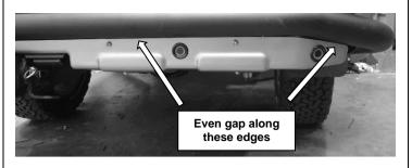
60. Position each diffuser panel so there is an even gap between the panel and the RSTB tube. Tighten fasteners to the specified torque.
