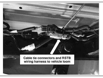
20. Connect the RSTB wiring harness to the 2 male 6-pin connectors.
