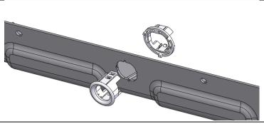
56. Push the sensor housing into the diffuser panel and then press the housing retainer on the rear until it firmly clips into place.
