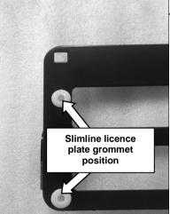
Insert 4 plastic grommets into number plate frame to suit licence plate size
