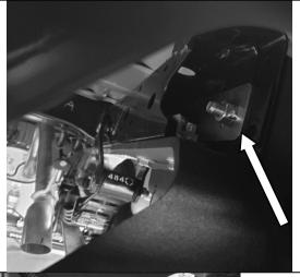
46. Fix the vertical plates of the RSTB to the chassis plate from fitting kit in each chassis rail using 3x M12x1.25x40 (fine pitch) hex head bolts, 3x M12 flat washers and 3x M12 flat washers per chassis rail. Leave finger tight at this stage as shown.
