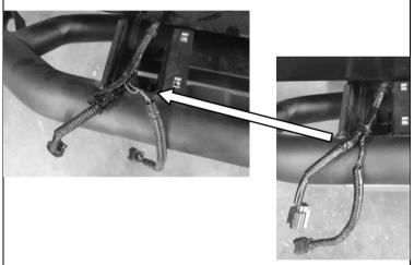
62. If the sensor loom is tight open up the conduit at the intersection of the two sensor wires exposing 50mm of sensor wires as shown. This can be done by removing a section of existing tape or carefully cutting the tape along the conduit join. Tape up exposed wires.
