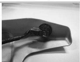
58. Clip the outer sensor into the housing as shown
