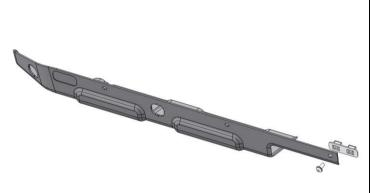
52. Fit the diffuser mount plate with M6 cage nuts, M6 x 16 M6 stainless steel button head screws and M6 flat washers to either the LH or RH diffuser as shown.
