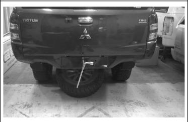
4. Remove the spare wheel from beneath the tub using the wheel nut wrench and jack handle pieces supplied with the vehicle. Insert as shown through the access slot above the number plate position and rotate counter-clockwise to release the wheel.
