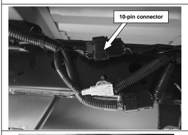
Locate the 10-pin connector on the left-hand chassis rail behind cross member as shown.
