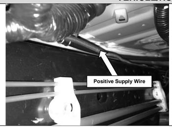
17. Route the positive supply wire to the front of the vehicle following the existing vehicle harness along the left chassis rail.
