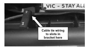
51. Tidy and fasten all wiring using cable ties and the slots in the RSTB brackets, as well as existing fastening locations.
