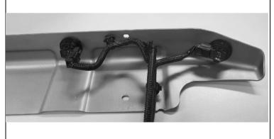
59. Sensor orientation on the LH diffuser panel must be exactly as shown. RH panel sensor orientation will be the opposite.
