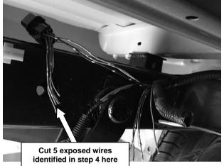
Warning: Wire colours may vary slightly and should be double checked with a multi-meter or test light. Failure to double check may result in damage to the vehicle.
