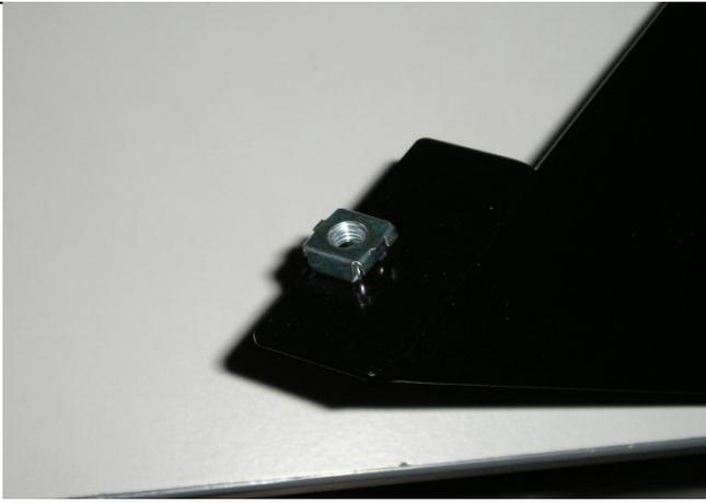
74. Fit M6 caged nuts to top surface of wing panels. Place the wing panels on top of the bottom lip of bulbar wing and secure using 6 x M6 x 20mm black bolts, spring washers and flat washers. Leave finger tight.
