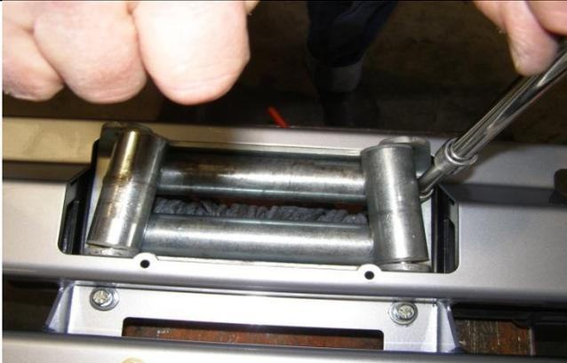
54. If circlips were removed, refit rollers and circlips after tightening bolts.
