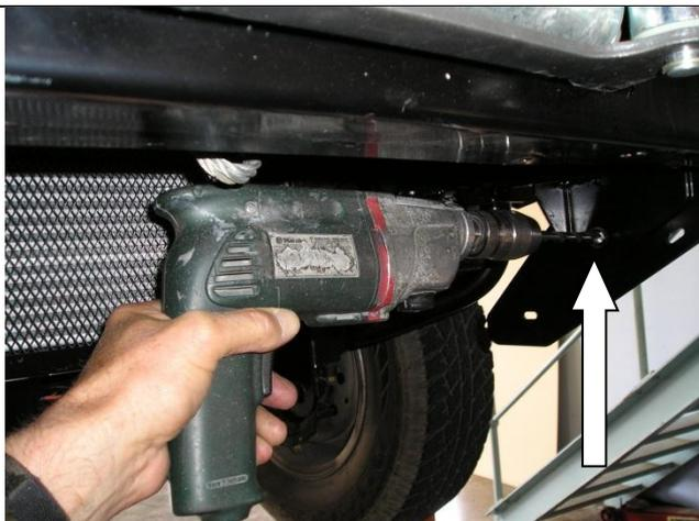
64. Using 10mm holes in pinning brackets as a template, drill through bar as per photo using a 10mm drill bit.
