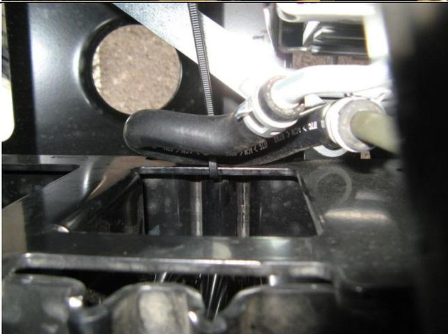
29. Secure transmission line to inside edge of chassis bracket using a cable tie supplied in kit.
