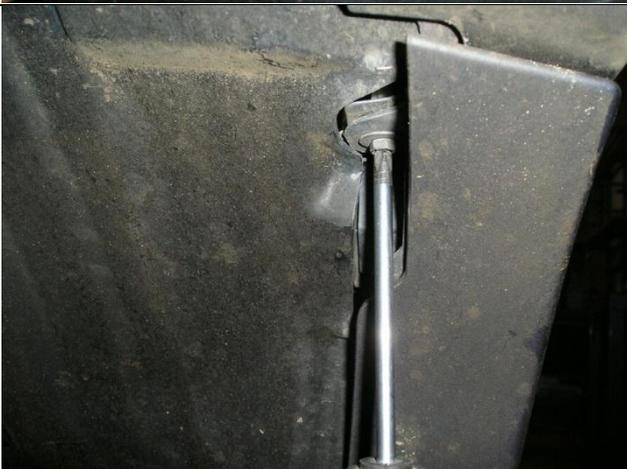
4. Remove vertical screws in wheel arch area holding wings of bumper onto fenders and set aside
