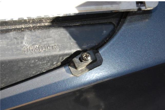
69. Fit light insert into bar. Secure using 4 screws, rubber washers and retainer clips from inside rear. ( Do not over tighten )
