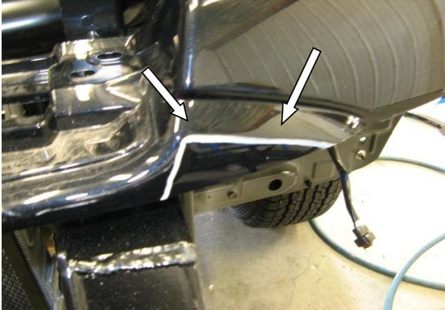
19. As in photo, mark a line as shown on both sides of bumper and cut away. This is to gain clearance for the bar upright. De-burr all edges.
