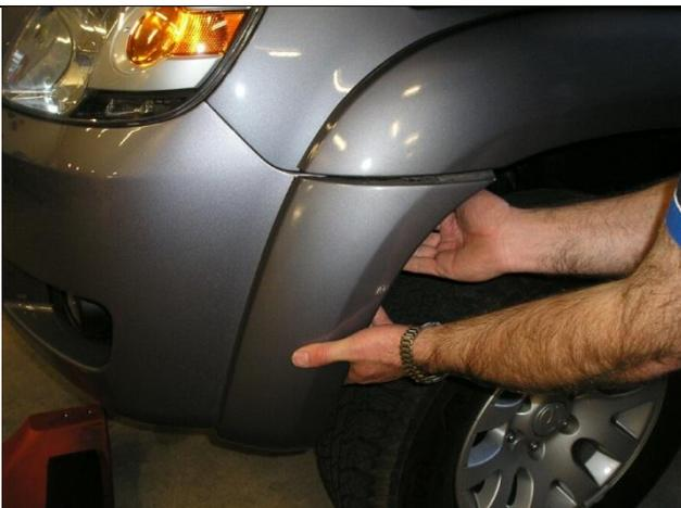
10. Pull outer wings of bumper as shown, when both sides are released carefully remove bumper and place on soft surface to prevent damage.
