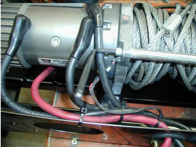
58. Pass cables through rubber grommets and connect as per Warn installation instructions. Fit plastic boots over terminals. Cable tie cables to bar as per photo to clear all moving parts.
