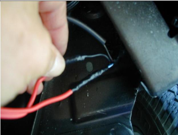
42. If vehicle comes fitted with fog lights, you must modify the O.E loom.
