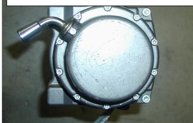
47. Stand winch upright and undo the cap screws and by lifting the gearbox only a couple of millimeters, rotate the gearbox. Once in position, refit all screws and tighten firmly.
