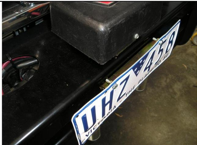
76. Fit number plate to number plate bracket using M6 hardware.
