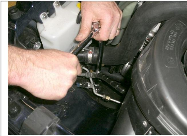
22. Using a long extension bar setup, undo vertical bolts holding crash bar from inside the engine bay, one is located next to battery the other on LHS as shown
