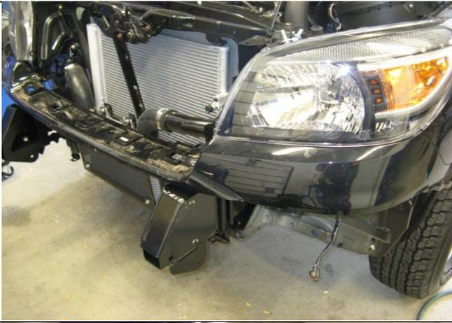
17. Once cut is completed use a file to de-burr the cut edges.
