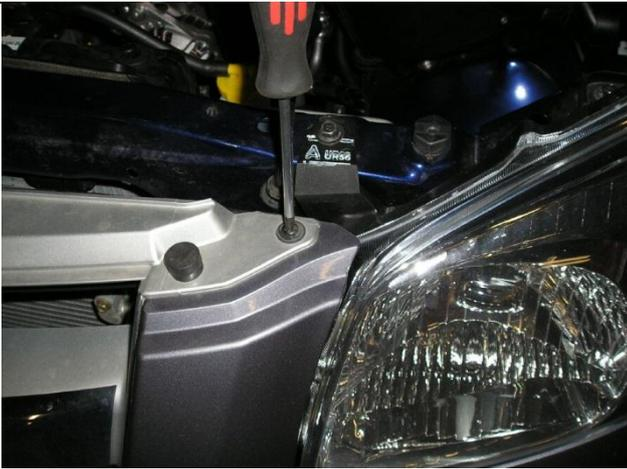
6. Remove screws holding grille in place
