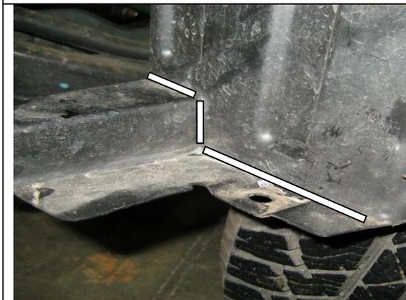
38. Unbolt the lower edge of the inner guard from vehicle. As per photo cut the forward facing lip from inner guard. Place inner guard up against sheet metal and mark position of the original M6 stud. Drill a 7mm hole in the inner guard and secure using M6 x 20 black bolt, black M6 flat washer and original M6 flange nut.
