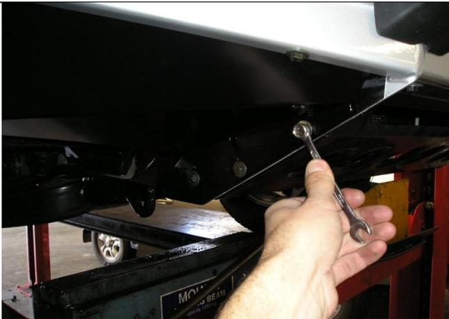
75. Secure wing panel to centre air deflector using 4 x M6 x 30mm black bolts, spring washers and flat washers. When everything is in place tighten all bolts.
