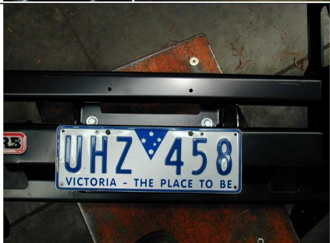
78. If the bar is a non winch bar setup, the number plate is fitted to front of bull bar directly as per photo using press in 2 x large round head plastic grommets and black Philips drive pan head screws. This position will cover the roller fairlead cutout in pan.
