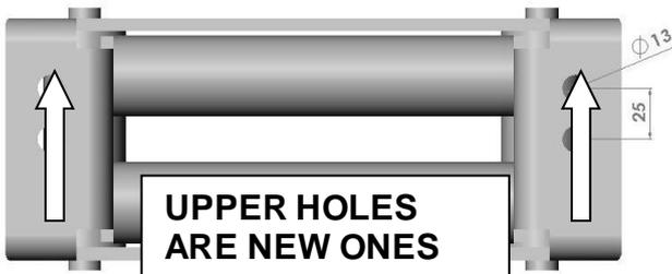
51. If necessary, mark out and drill two new 13mm holes in the roller fairlead, 25mm apart from the original holes, as shown on the adjacent picture.
