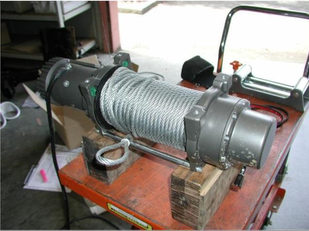
48. An ideal method to fit a winch into bar is to pack winch up on a bench to enable you to lower bar down on winch
