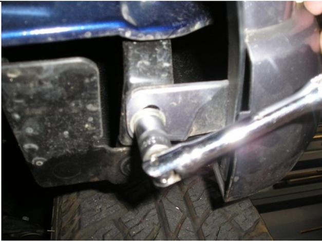
1. Remove screws and plastic scrivets holding lower bumper in place and set aside
