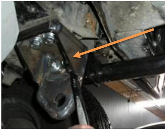
34. Attach lower mounting bracket to LHS brace / recovery point using 10mm hardware.
