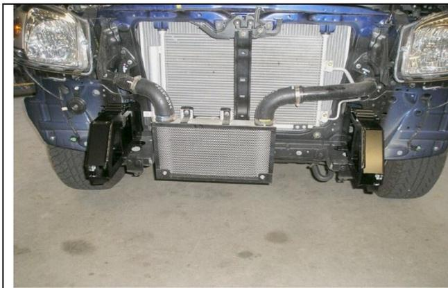
37. With impact absorbers fitted and tightened check that the inside measurement across the faces is 815mm
