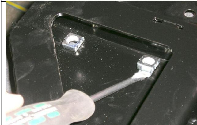
24. Fit M10 cage nuts to impact absorbers as shown, use a screwdriver to assist pushing in flange.
