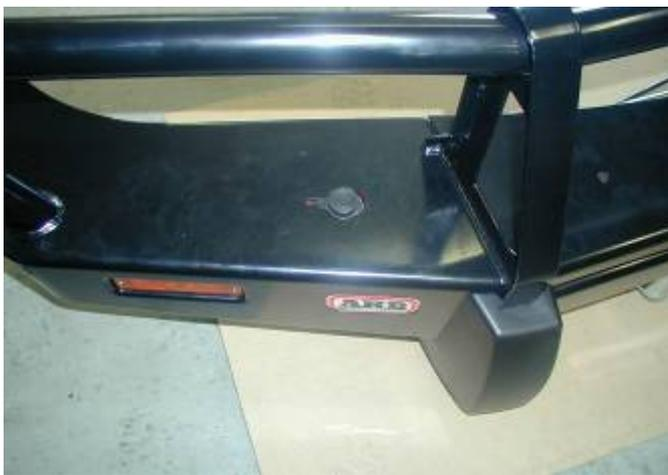
11. When the control box is secured to the bull bar, adjust the control box so that the remote cap is central in the cutout in the wing. When satisfied tighten the control box to control box bracket bolts and the control box bracket to bull bar bolts.
