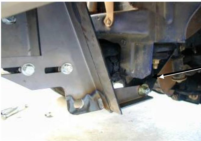
19. Secure the lower bull bar mounting holes to the vehicle tie down plates using M12 x 35mm bolts, heavy-duty flat washers, spring washers and 12mm nuts. Tighten bolts until the heavy-duty washers deform.
