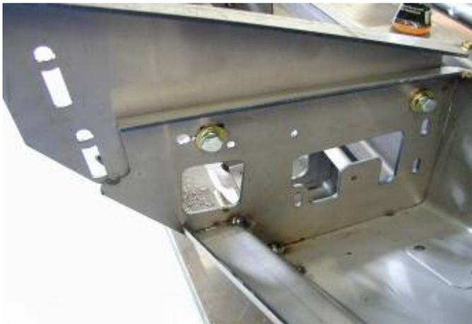
16. Attach the impact absorbers to the bullbar using four M10 x 30mm bolts, M10 nuts, M10 flat and spring washers Do not fully tighten the bolts at this stage.
