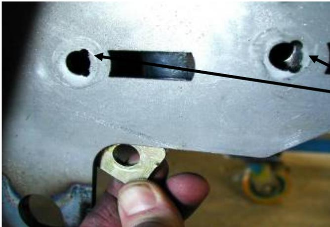
18. Using the assistance of two people, position the bull bar over the chassis rails. Insert the square 4mm washers between the chassis and the impact absorber and fix in place using four M10 x 40mm bolts, M10 flat and spring washers. Tighten bolts.
