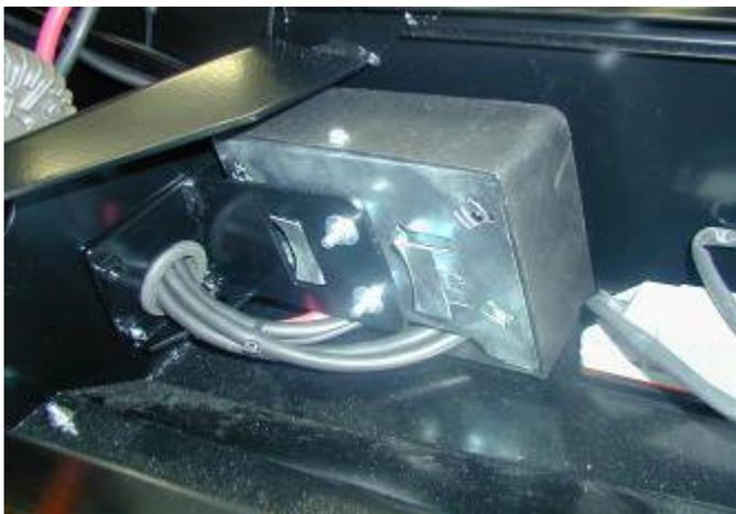
9. Fit the control box cables through the rubber grommet of the control box bracket and cable tie together.
