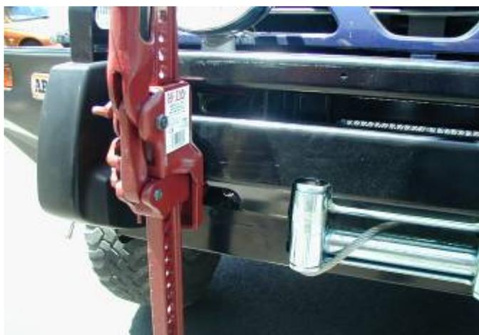
Mounting holes for the use of a high lift jack have been incorporated on both sides of the bull bar.
